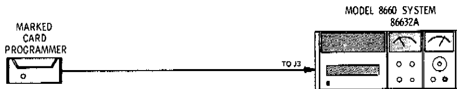
Figure 4-6. Remote Programming Test Setup
